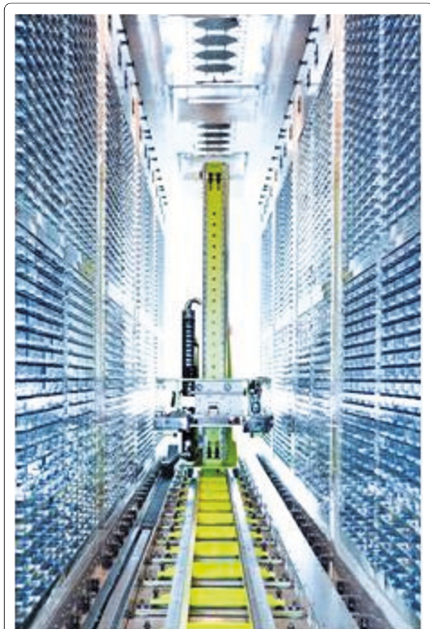
Figure 2. Sample storage and aisle robotics used to archive and retrieve samples in UK Biobank. Samples identified by individual barcodes are held in automation compatible racks at -80^{\circ}\text{C} in independent storage towers maintained at temperature by liquid nitrogen circulating in a closed evaporator system. All sample transfer and retrieval processes are automated to ensure accuracy and speed.
